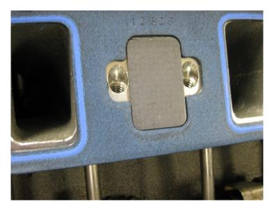
**STEP 11:** Rub an initial thin layer of silicone onto the end rails of the intake manifold <u>and</u> block.
