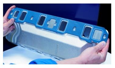
**STEP 2:** Inspect intake manifold for debris, and make sure it's clean. Check all threaded holes and tap deeper if necessary. Check the carburetor/throttle body gasket alignment. Also look at the gasket surfaces for nicks and damage, raised surfaces on the flanges can impede sealing.
