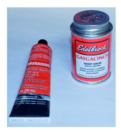
**STEP 9:** Apply a thin coating of Gasgacinch on the head intake port flange and the head side of the intake manifold gasket. Within a few minutes, the surfaces will start to dry and become tacky. Carefully place the gaskets on the head surface aligning ports and bolt holes.
