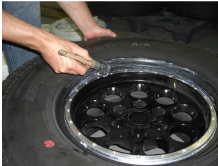
Pic 3.1 – Apply a liberal amount of tire soap to the entire bead.
