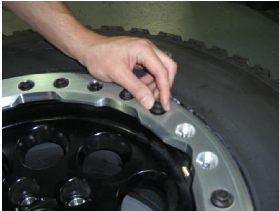
Pic 5.1 – Hand thread in all remaining bolts.
