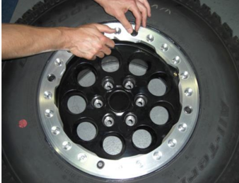
Pic 4.1 – Hand thread 4 bolts at the corners.
