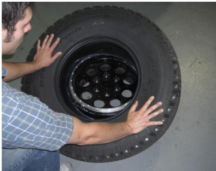
Pic 1.1 – Force the inner tire bead over wheel flange
