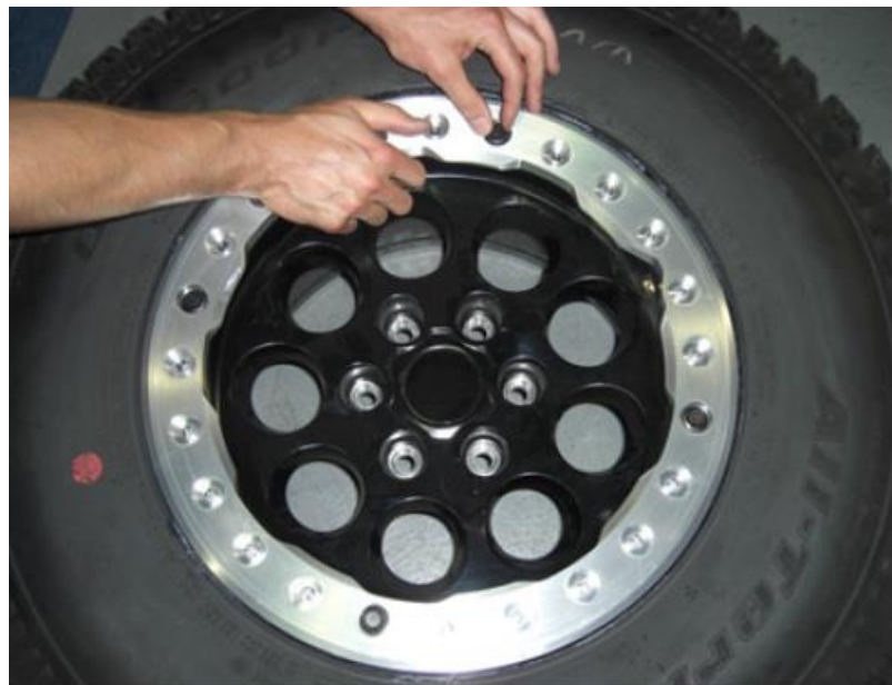
Pic 4.2 – Tighten each bolt at least 1 full turn with a socket wrench
