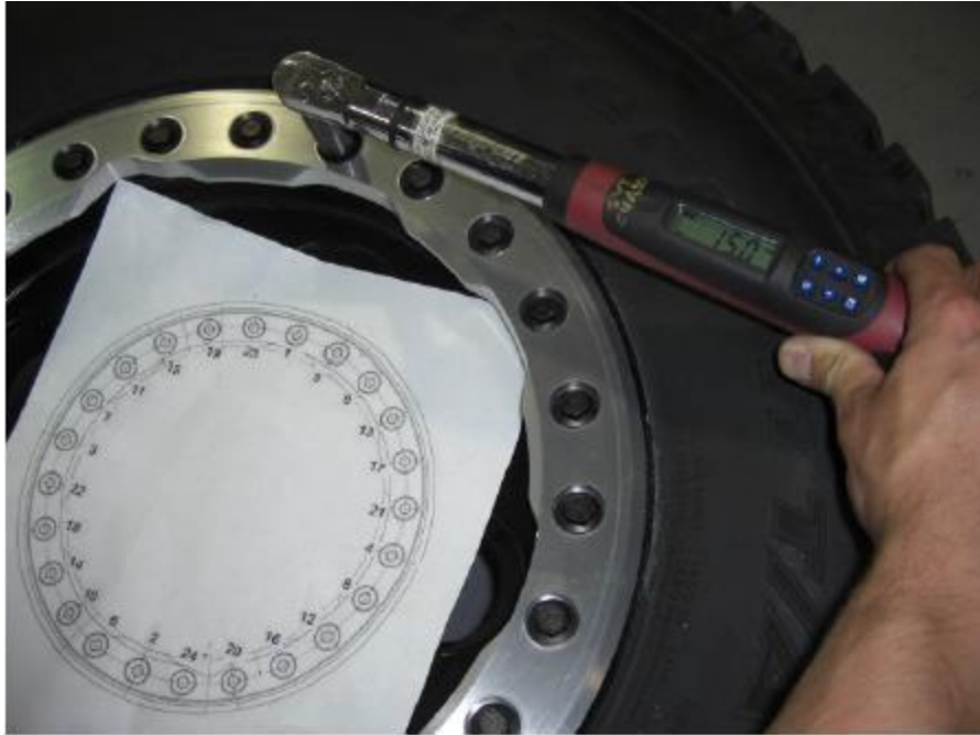
Pic 6.2 – Torque in the proper sequence using a torque wrench.
