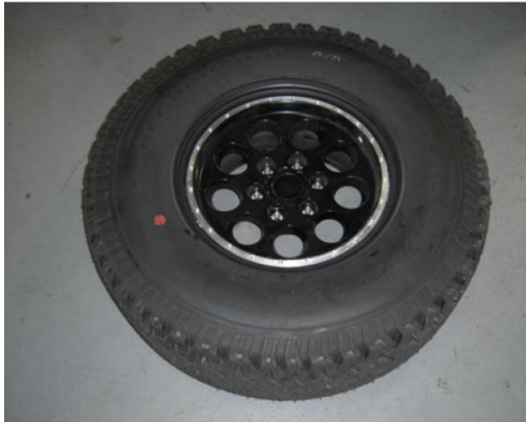
Pic 2.1 – Outer tire bead fits on wheel flange
