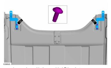
2. To install, reverse the removal procedure with the provided Z-brackets.
