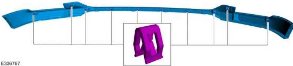
5. Remove the bolts and the pin-type retainer. *Torque: 36 lb.in (4.1 Nm)*
