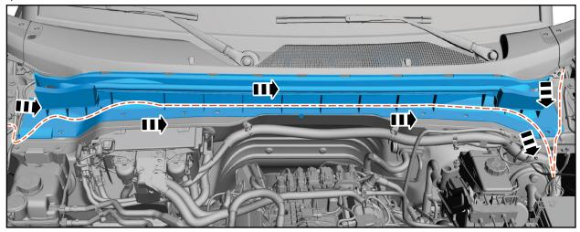
10. Splice the power wires to the VT-GN blunt wire (one of the 6 blunt wire leads bundled together).
