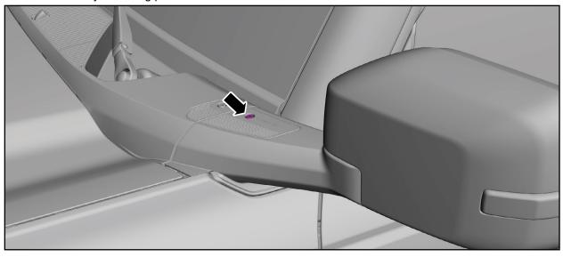
2. Position the RH and LH spot-lamp mounts and install the bolt and washers, do not tighten yet.
