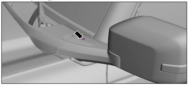
2. Position the RH and LH spot-lamp mounts. Apply Loctite 242 Removable Medium Strength Blue Threadlocker or equivalent to the flange head chrome bolt and install, do not tighten yet.
