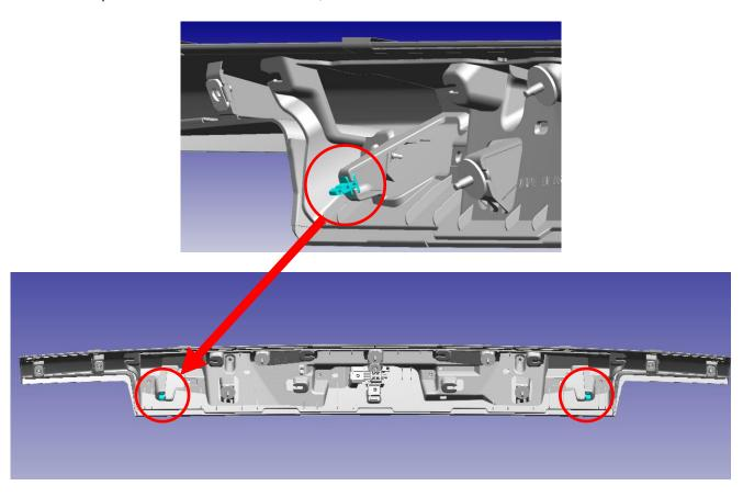
14. Install a tub clip onto the trim pins on both sides.
