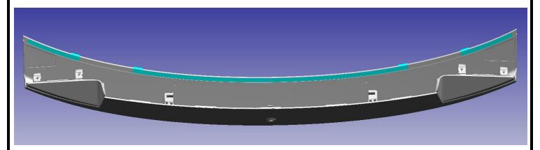
5. Place the inner module into the outer spoiler module. Make sure the inner module clips in on both sides. RH side shown, LH side similar.
