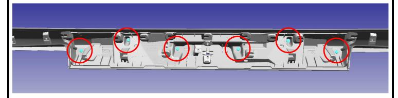
7. Remove the protective backing from the clip foam and install as shown below.
