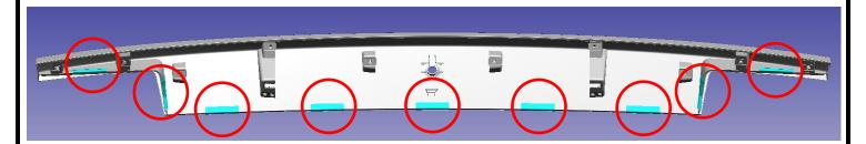
3. Remove the brown protective backing from the foam rectangles and install to the outer spoiler module.
