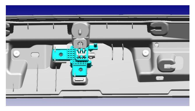
12. Use two screws to secure the camera housing.
