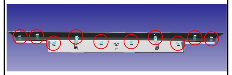
2. Remove the red protective backing from the nine rubber seals and install to the outer spoiler module.
