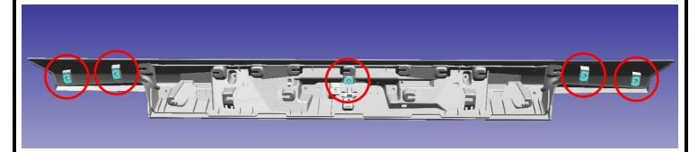
8. Install five T-studs with foam to the spoiler module. Make sure T-studs clip in.
