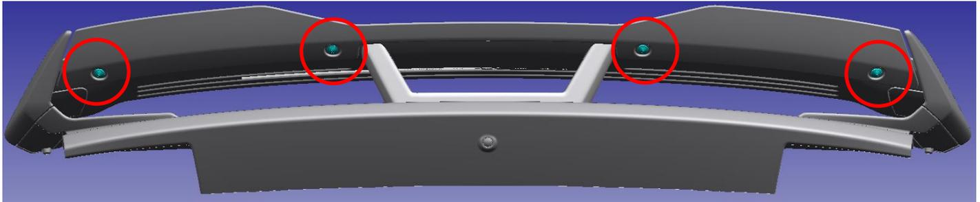
13. **NOTE:** When installing the spoiler, apply approximately 15 lbs. of pressure along the length of the spoiler to ensure adhesion of the two-side tape.
