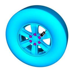
Install the wheel and tire and install the wheel nuts.
