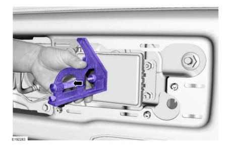
Keeping the combination square level on the face of the <u>CCM</u>, adjust the pitch by using an E6 Torx® socket to adjust the screws until the CCM is vertical and level.
