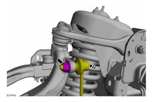
Install the new upper ball joint nut. *Torque*: 46 lb.ft (63 Nm)
