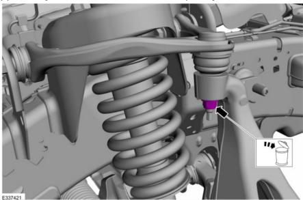
NOTE: Be sure not to damage the ball joint boot when installing the Ball Joint Separator.
