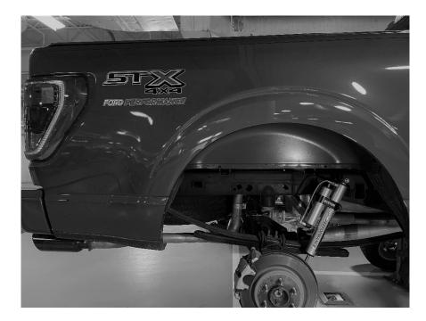
Install the new rear shock absorber upper and lower bolts and nuts. *Torque*: 66 lb.ft (90 Nm)
