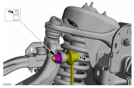
Remove and discard the 2 shock absorber and spring assembly lower nuts.
