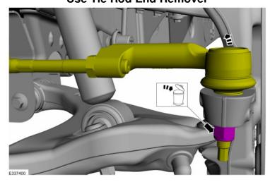
Remove the brake hose bracket bolt and position the brake hose bracket aside.
