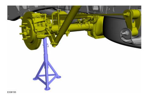
Remove and discard the rear shock absorber upper and lower bolts and nuts. *Torque*: 66 lb.ft (90 Nm)
