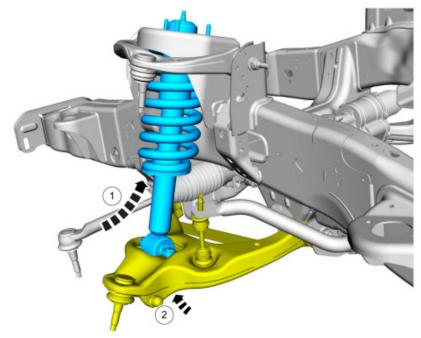
Install the 3 new shock absorber and spring assembly upper nuts. *Torque*: 52 lb.ft (70 Nm)
