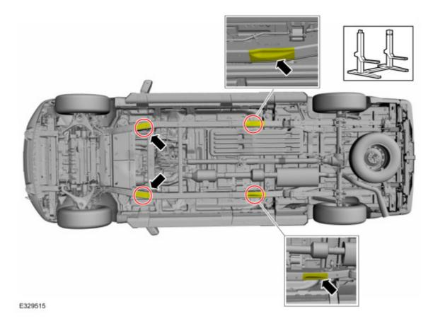
Refer to the picture above to find the appropriate jacking points: Note this works for all F150 vehicles, Hybrid, 2WD or 4WD.
