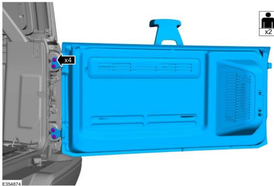
10. Mark the location of the tailgate hinge bracket to aid in installation.
