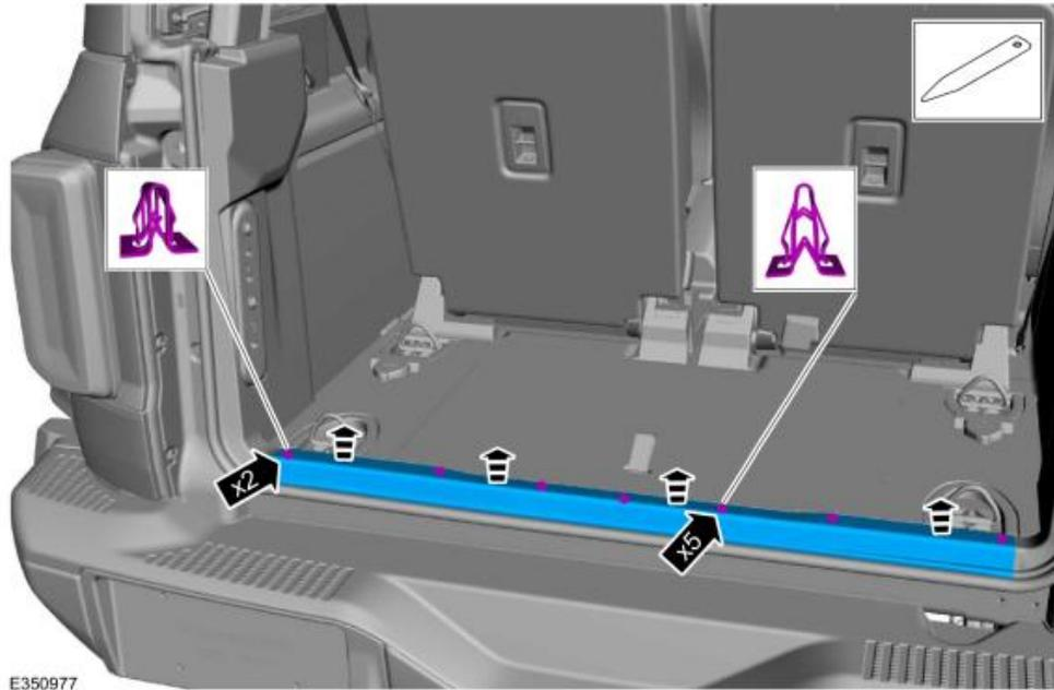
4. Pull the rear edge of the load space trim panel enough to detach the tailgate wiring harness electrical connector.
