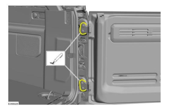
8. Remove the clip holding the tailgate strut and position aside.
