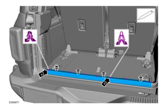
4. Pull the rear edge of the load space trim panel enough to detach the tailgate wiring harness electrical connector.
