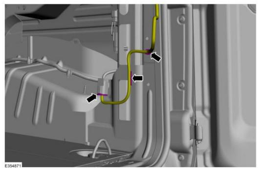
6. Remove the fasteners and the tailgate hinge cover.
