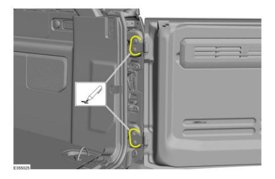
8. Remove the clip holding the tailgate strut and position aside.
