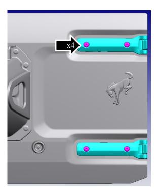
12. Remove the fasteners and rubber bumper spacers.
