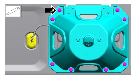
4. Remove the fasteners and rubber bumper spacers.
