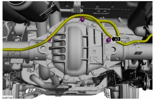
To drain fluid, losen bolts and studs slowly. Once drained, remove bolts and studs to remove cover.
