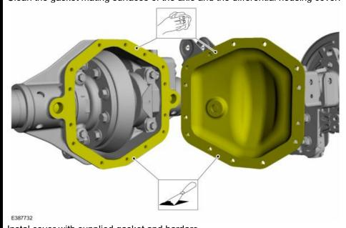
Instal cover with supplied gasket and hardare.
