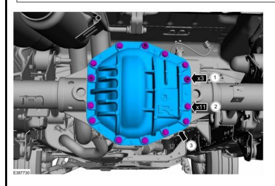
Clean the gasket mating surfaces of the axle and the differential housing cover.
