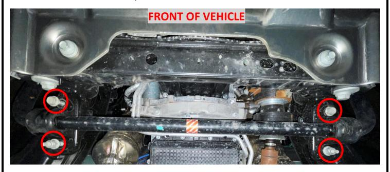
4. On both sides, install the sway bar brackets provided with the kit underneath the sway bar then reuse the bolts from the last step and tighten.
