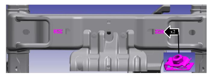
4. Attach the skid plate brackets to the frame using the bolts and washers (M10x35). (left side shown, right side similar)
