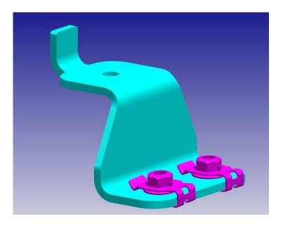
2. On both sides, attach the frame J-clips to the frame with the nut side of the clip facing into the frame. Cross section view shown for reference. (left side shown, right side similar).
