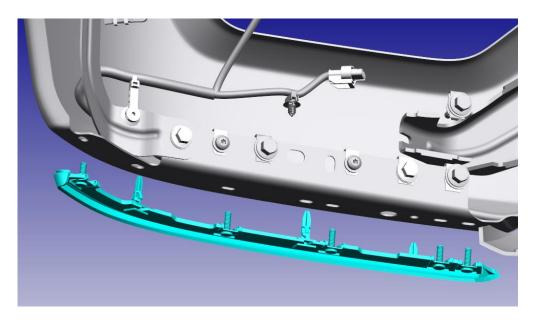
2. Secure the lower valence bumper cover to the bumper reusing the M6 nuts (left side shown, right side similar).
