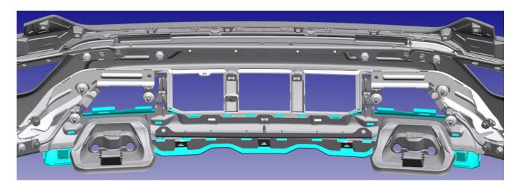
4. Secure the kit bumper cover using the bolts and washers (M6x25).
