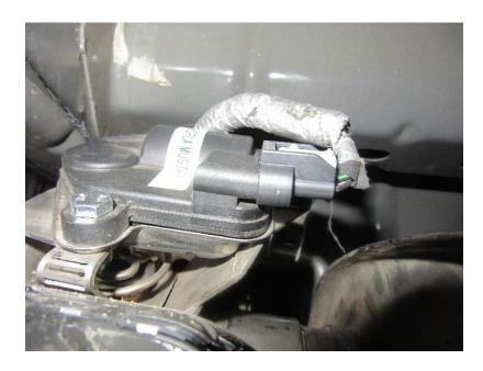
STEP 4: Using a 15mm socket loosen nuts on clamps at the front of the factory System.
