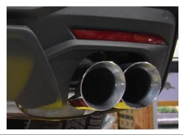
Step 7: Check your exhaust system for proper clearance under the vehicle and also for tip alignment, tighten the clamps to 48 Nm (32-35 ft. lbs), checking tip alignment and clearances as you do. There should be a minimum gap of 25mm from the tips to the edge of the car, and the tips should be in 25mm from the outermost edge of the rear bumper.
