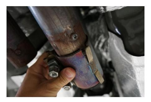
Step 2: Install new front muffler (x-pipe) onto clamps. Snug but do not tighten.
