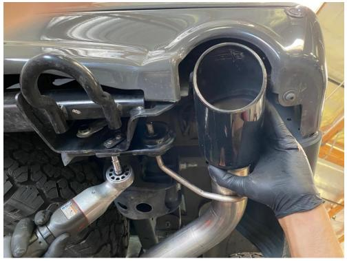
Step 5: Slide a clamp over the expanded inlet of the crossover pipe and slide onto the overaxle pipe. Do not tighten the clamp.
