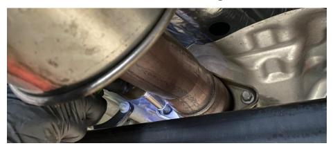
STEP 7: Slide the assembly backwards to remove the hangers from the isolators, then tilt down and remove forward.
