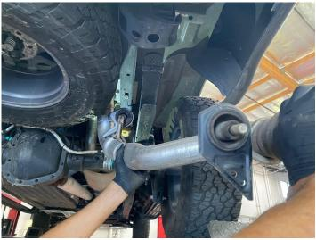
STEP 5: Work the tailpipes out of the expanded muffler outlets and around the spare tire. Pull off the isolators to use with the new exhaust.
