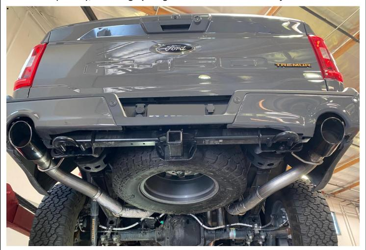
STEP 8: Start vehicle and check for any leaks. If any leaks are found, determine cause (such as loose or incorrectly positioned clamp) and repair as necessary.
