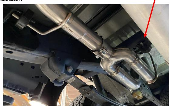
Step 4: Slide a clamp over the inlet of the RH tailpipe, and slide the tailpipe over the overaxle pipe. Then slide the isolators onto the hangers. Attach the isolators to the frame using the factory bolts. Do not tighten the clamp.
