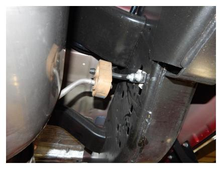
STEP 3: Slide a clamp over the tailpipe inlet. Install the tailpipe by working it over the rear axle and sliding it onto the muffler outlet pipe.
