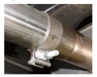
Step 6: Adjust tips to the side of the truck, with minimum  $\frac{1}{2}$  gap on top of the tips.
