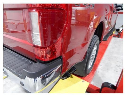
Step 7: Once you are satisfied with your fitment torque all clamps to 48 N.m. (35 lb-ft). Check clearances to wires, brake lines, and body parts.
