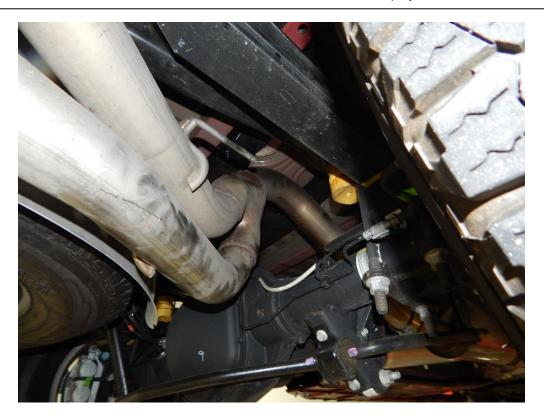
STEP 4: Slide the rear-most isolator removed earlier over the hanger of the tailpipe assembly and attach to the frame. Torque the bolts to 22 ft-lbs (30 N-m).
