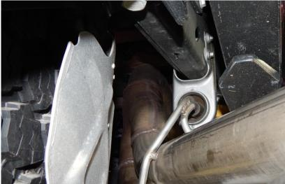
STEP 6: Slide the muffler and tailpipe rearward off the front pipe and out of the isolators behind the large muffler. Then slide forward and down to remove, rotating as necessary.
