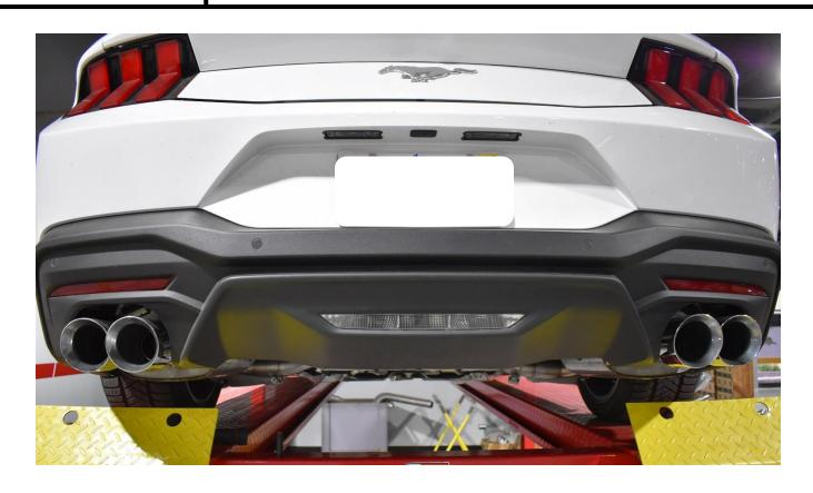
STEP 8: Start vehicle and check for any leaks. If any leaks are found, determine cause (such as loose or incorrectly positioned clamp) and repair as necessary.
