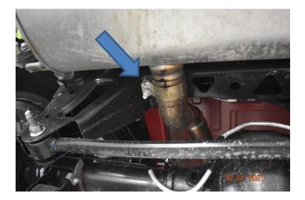
STEP 3: Lubricate all hangers shown below, pull off factory muffler hangers.
