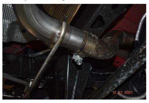
STEP 2: Place the hanger bracket over the studs of the factory bracket and attach using the nuts supplied.
