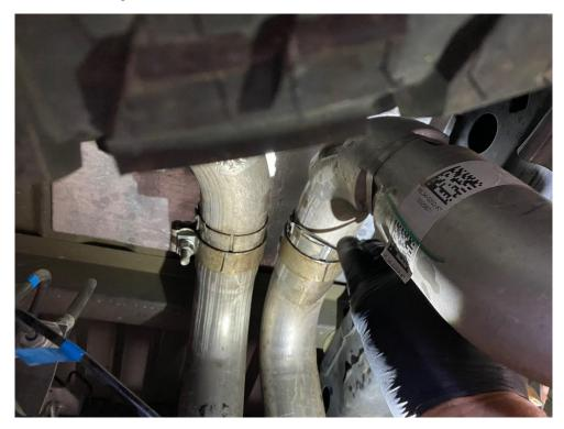
STEP 6: Remove the 2 bolts from the front flange. Save for re-installation.
