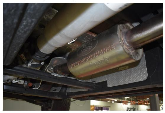
STEP 2: Slide a clamp over the expanded inlet of the intermediate pipe. Slide the assembly over the front muffler assembly outlet and push the hanger into the rubber isolator.
