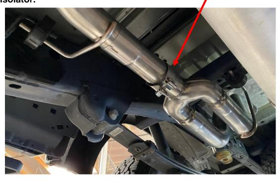
Step 4: Slide clamps over the inlet of the tailpipes, and slide the overaxle pipes Into the tailpipes pipe. Do not tighten the clamps.
