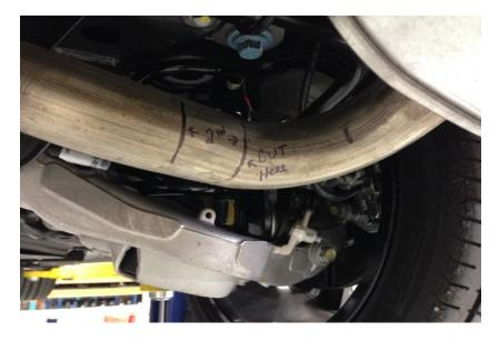
Passenger side muffler (Cut line is the start of the bend going into the muffler)
