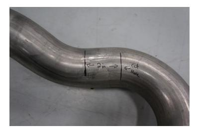
STEP 4: After cutting is completed remove muffler from rear hanger, deburr intermediate pipe. For vehicles with valves, disconnect the valves at the rear mufflers (LH and RH). Pull the pin holding the connector in, slide it out of the valve actuator assy.
