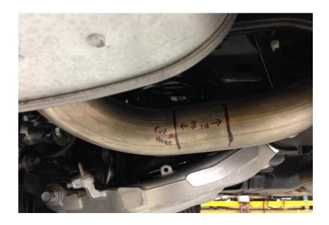
Drivers side muffler (Cut line is the start of the bend going into the muffler)
