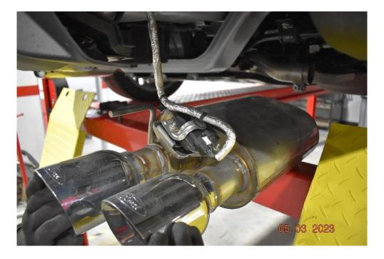
STEP 2: Install drivers side muffler into rear hanger slide clamp onto muffler pipe, slide muffler onto the pipe that you just cut. Position tips in bumper cutout and torque clamp to 48Nm (35 lb-ft).
