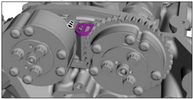
Activate the secondary timing chain tensioner by pressing down on the secondary timing chain and tensioner top shoe until it bottoms out, let go of the tensioner and it will spring up putting tension on the chain.
