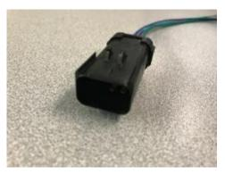
The 6-way pigtail is to be connected according to the chart below. See also the diagrams on the following pages for illustrations of wire connection points, based on the ignition/starter switches that you intend to use. Setup A uses separate toggle switches for ignition and starter inputs, while Setup B uses an ignition cylinder with a key.
