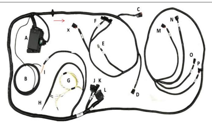
Figure 1a - 2020 7.3L AUTOMATIC CONTROL PACK MAIN HARNESS
