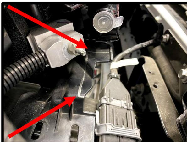
92. Install the supplied pump mount bracket frame opening on **LH** side. Slide J-nut through opening on frame. Secure bracket to J-nut using supplied (1) 6mm x 30mm HHFCS. Install pump clamp to bracket using the supplied (2) 6mm x 10mm HHFCS bolts. Mount pump in clamp using the 1" wide rubber strip around pump, secure clamp. **NOTE:** Outlet fitting should be facing straight up, inlet should be facing center of vehicle.
