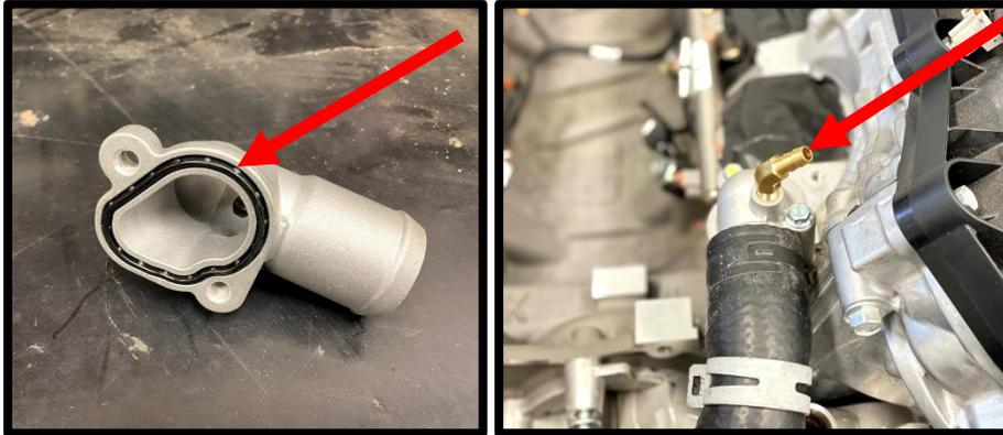
31. **(Single Alternator)** Reinstall water neck hose to new water neck. Using needle nose pliers, reinstall and rotate the factory pinch clamp at the water neck towards the driver side for future clearance of the SC. **NOTE:** Image shows clamp with SC installed to illustrate max clearance.
