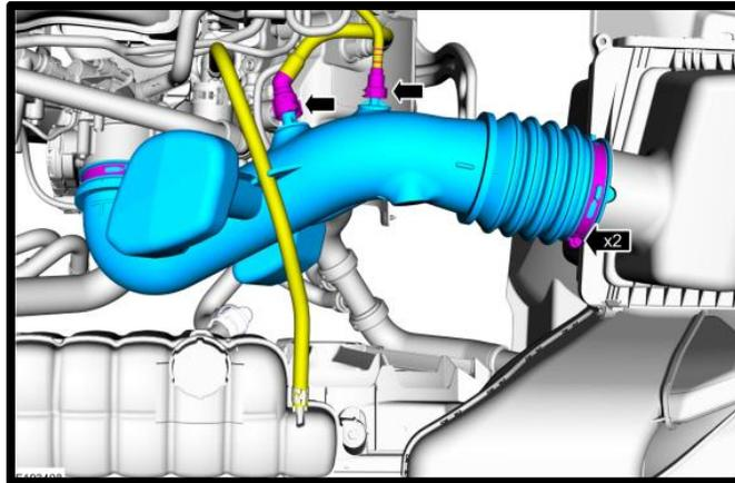
14. Using a 13mm socket, remove the (1) factory fastener securing airbox to the fender. Using a panel pulley or flat head screw driver, remove the (2) push-pins from the factory air snorkel. Remove airbox from vehicle.
