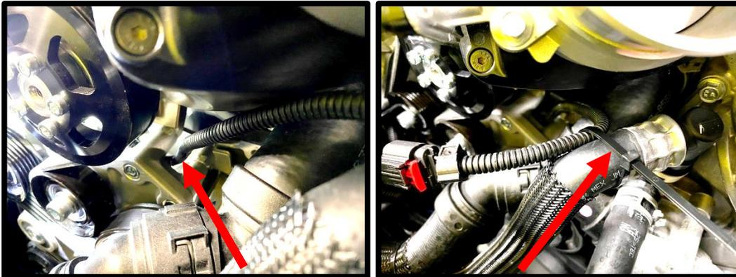
71. Reinstall the water pump pulley using a 10mm socket, torque to 14 lbs-ft.
