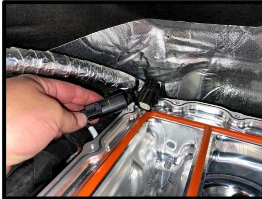
70. Install the supplied electronic throttle pigtail to the factory electrical connector. Route under front idler plate front support for proper safety from belt. Push until it locks in place, then lock the safety lock. Route to **LH** side of vehicle for later connection to throttle body. **TIP:** When pressing together, hold the wires vs connector to ensure the wires do not come loose during connection.
