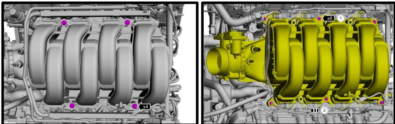
21. Use compressed air and remove any direct or foreign material from cylinder head, block and surrounding area of the fuel rail and injectors. Remove the intake manifold from the engine. To do so, remove the (5) wire harness push pin supports from the back of the intake manifold and disconnect the 4-way MAP sensor connector.
