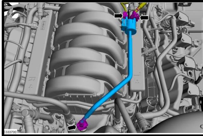
17. Carefully remove the factory fuel line by releasing the safety lock, then squeezing the connector and pulling back. The fuel system may still have pressure, use protective eyewear and multiple rags to catch any possible fuel leak. **NOTE: THIS FUEL LINE HAS A CHECK VALVE, DO NOT FLIP ORIENTATION. DO NOT REMOVE FROM DI PUMP TO ELIMINATE CONFUSION. 90-DEG END ALWAYS CONNECTS TO FUEL FEED SUPPLY!**
