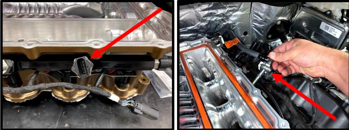
76. Slide the EECPV to previously installed bracket. Connect factory plastic quick connect fitting to EECPV until it clicks and locks into place. Connect 2-way electrical connector to EECPV, press locking tab back in place.
