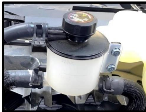
119. Cycle the ignition to the ON position again and repeat until the sound of the electric pump is continuous without any pulsation and the fluid level is met at the filler cap. **NOTE: During water pump start-up, it is normal for a slight pulsation to occur. Once the pump has reached its maximum cycle speed, no pulsations should be present. If any pulsations occur, there is air in the system. NEVER GO WOT UNTIL AIR IS BLED OUT!**
