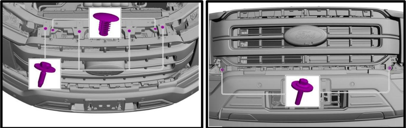
11. Remove the (4) pin-type retainer. Pull up and disengage the locating pins along the top of the grill. Pull forward on center of the grill to remove.
