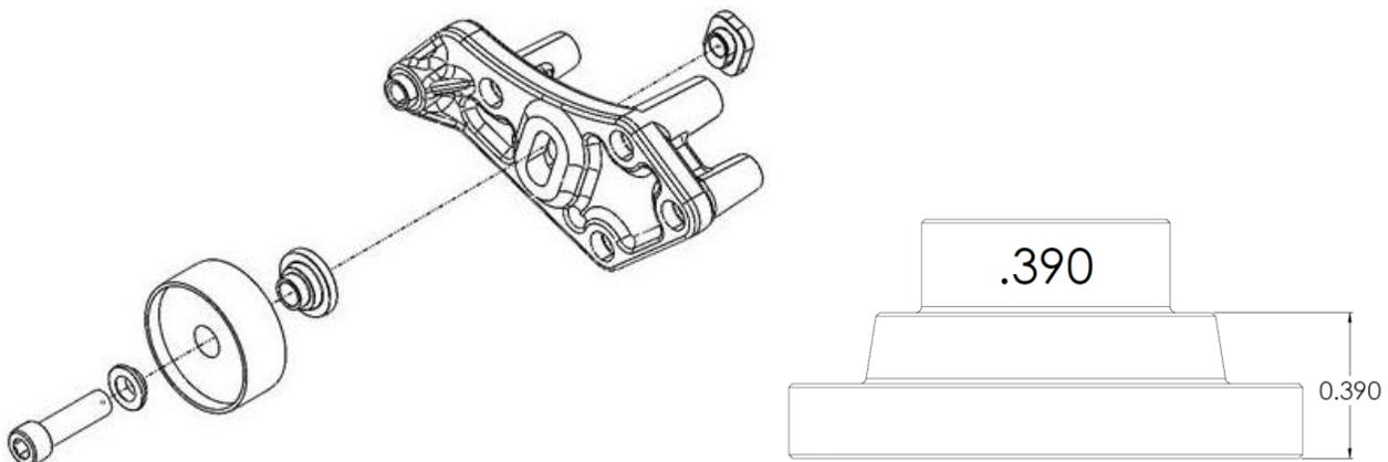
81. Install the supplied (1) grooved idler pulley #36326 to the idler plate using the (1) idler step washer and (1) ½"-13 x 2" SHCS. Install the supplied circulating pump bracket under ½" bolt head, secure other end to front engine timing cover using stock bolt. Torque idler pulley bolt to 30 lbs-ft. using a 3/8" allen socket. Use light amount of anti-seize on threads. **NOTE: Some models are built without these pumps, if so, discard this bracket.**
