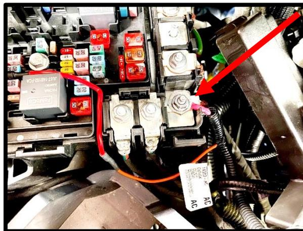
110. Remove the ground bolt from the **RH** side frame, next to the battery using an 8mm socket. Install IC pump relay ground eyelet here. Secure with factory bolt using an 8mm socket.
