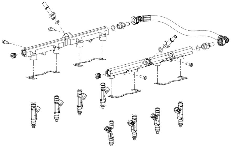
54. Apply generous amount of grease to the injector orings for ease of installation. Install the fuel injectors, rails and lock bracket to the intake manifold, secure with the (4) 6mm x 16mm SHCS using a 5mm allen socket and use **Blue Loctite #243**. Torque to 90 lbs-in.
