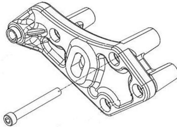
66. Torque the (10) 6mm (10) HHFCS manifold bolts in the following pattern using a 10mm socket. First pass: 88 lbs-in. Second pass: 106 lb-in. **NOTE:** For bolt #10, a 1/4" socket with 4"-6" extension, 10mm wobble is the best possible tool to get into this tight area.
