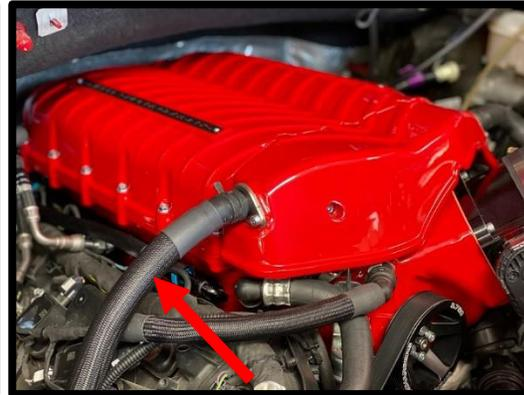
98. Install throttle body adapter to supercharger inlet using the stock bolts using the supplied gasket between TB adapter and SC inlet. Torque to 89 lbs-in. Install the stock throttle body using the (4) stock bolts using a 10mm socket.
