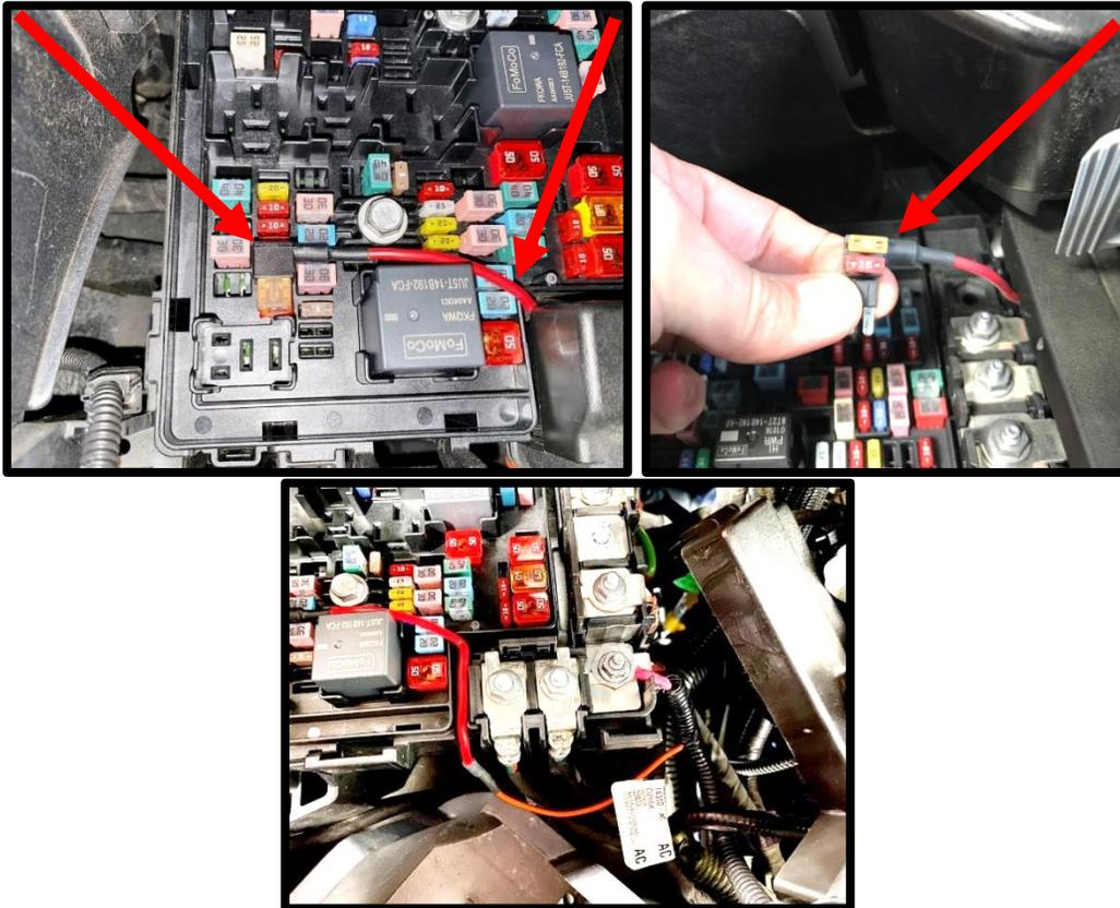
112. Install the fuse box cover, ensure the turn-on wire is clear of cover.
