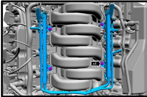
23. Disconnect all 8 fuel injectors from factory injector harness.
