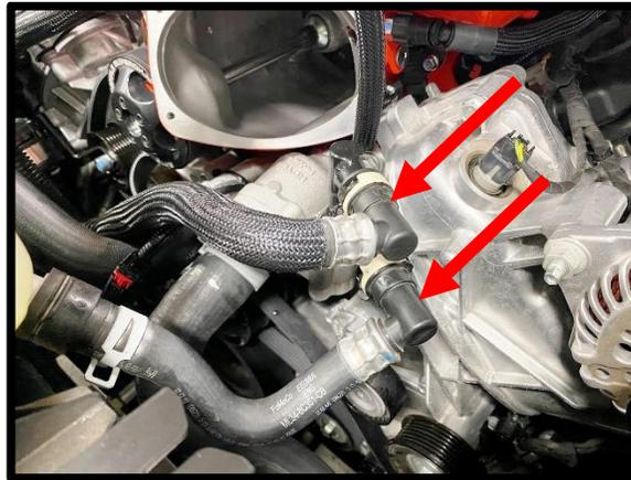
43. Using masking tape or similar, wrap around 4-way TMAP sensor connector, you will connect the extension to this after SC installation and it will be easier to find.
