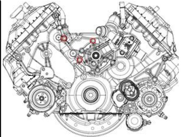
48. Use the supplied (3) 8mm x 90mm SHCS to secure the idler plate to the engine. Using a 6mm allen, torque to 22 lbs-ft.
