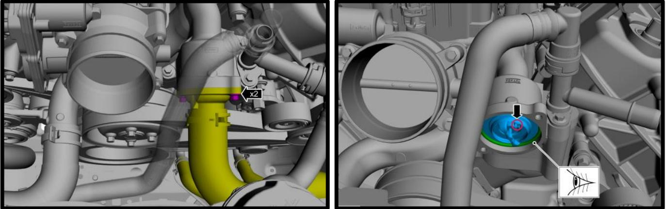
37. **(Dual Alternator)** Install the factory thermostat and thermostat oring to new housing. Install coolant inlet using the factory (2) bolts. Torque to 89 lbs-in.
