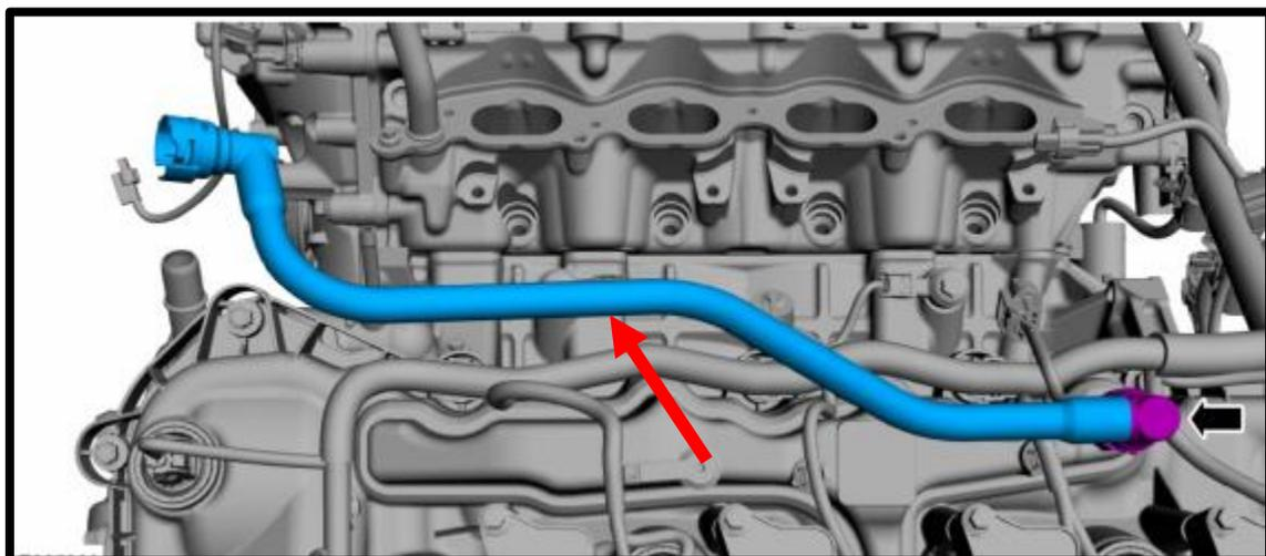
13. Disconnect the (2) quick connect fittings from air inlet tube. Using a 9/32" nut driver, loosen the factory hose clamp securing the air inlet tube to the throttle body and airbox. Carefully cut the electric tape securing the ETC wires to the throttle body. Disconnect the electronic throttle electrical connector by pushing up on the safety lock and then squeezing the connector and pulling away.
