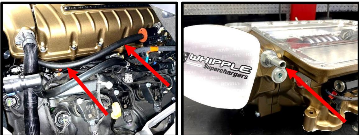
78. Install the stock PCV hose to the **RH** side valve cover. Connect other end to the supercharger inlet 15.82mm quick connect fitting. \*Note: This requires you to rotate the fittings for proper fitment. Push until it clicks and locks into place.
