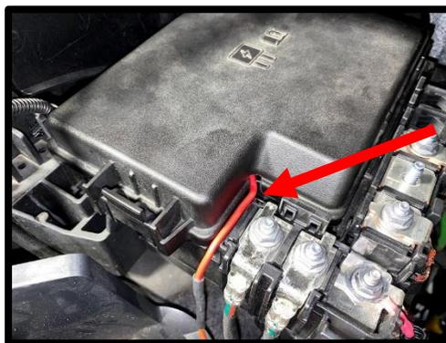
113. Secure the relay/fuse with zip-ties along with the harness for a clean installation. Route IC pump connector down below radiator, secure to IC pump previously mounted. Ensure all other wires are clear of the belt system, use zip-ties to eliminate any potential interference.
