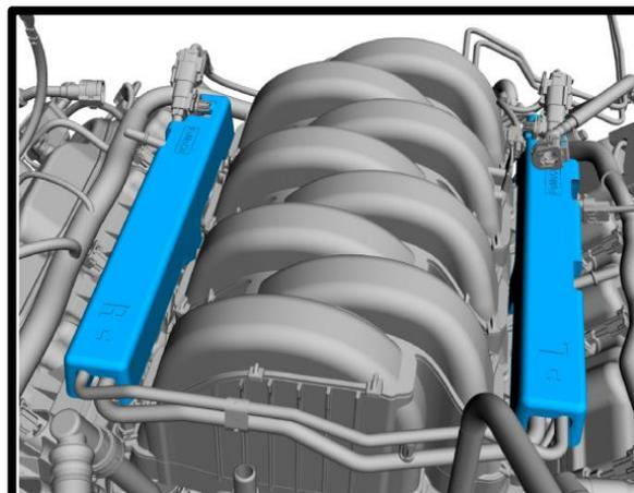
19. Disconnect the (2) injector harness 6-way pigtails and push connectors out of the way. Remove the fuel PSI sensor electrical connector from the driver side fuel rail by releasing the locking tab and squeezing connector, then pulling away.
