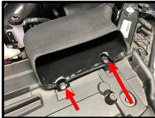
103. Install the supplied panel filter to the airbox lower. Install the upper airbox to the top of the filter. Secure the top to bottom using the supplied (6) 6mm x 16mm BHCS. Torque to 50 in-lbs. **\*Caution:** Over torquing can result in pulling an insert out of plastic box.
