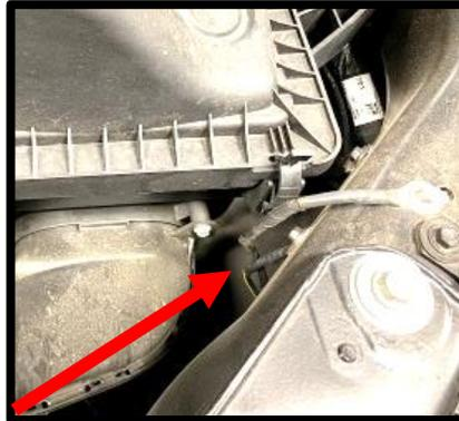
102. Install the supplied lower airbox into factory (2) hole locations. Using the supplied (2) 1.1" L x .30" W plastic push pins, secure front of snorkel to factory location.
