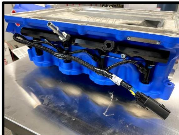
55. Install the supplied 1/4" ID bypass actuator to the bypass nipple and 1/4" 90deg nipple on SC inlet. **CAUTION:** Do not open/close bypass actuator by hand. This may damage actuator internally. It only moves properly with equal vacuum/boost at the actuator reference port.
