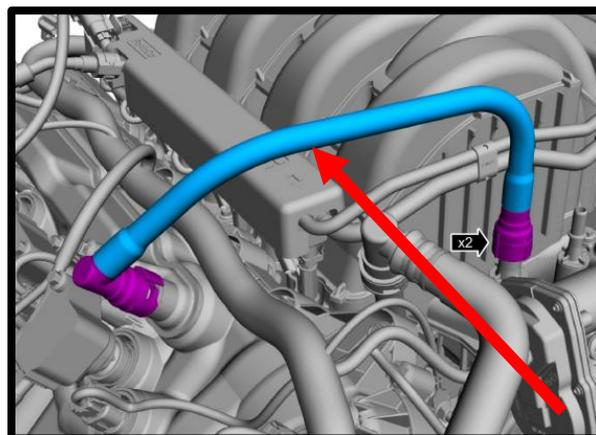
16. Disconnect the EECVP (EVAP) solenoid electrical connector by squeezing locking tab and pulling away. Disconnect the EVAP solenoid quick connect fitting hose from the EECVP solenoid and from the intake manifold by releasing locking tab and pulling away.
