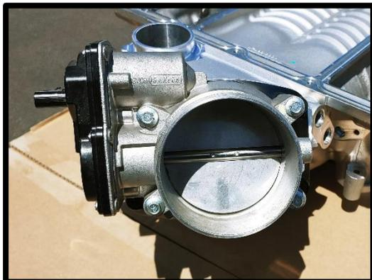
99. Connect the electronic throttle extension to the electric motor. Press until it clicks and locks into place. Press the safety lock until it clicks and locks into place. **NOTE: Secure harness with zip-tie. It should have some slack around connector for motor vibration, only zip-tie to avoid belt system.**
