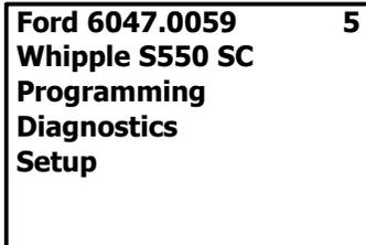
9. Once you're done flashing, cycle the key off for 5 seconds, then back on. Select the "**Diagnostic**" tab, read all the DTC (trouble codes). Erase all codes. Note: De-energizing relay code is common after flashing and will go off after a few driving cycles or if you hit clear DTC 5-6 times. The vehicle will run proper even if this code is on.
