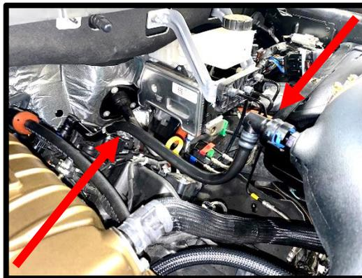
107. Remove the stock fuse box cover located near **RH** firewall. Using small file or cutters, make notch the box as shown for the power wire.
