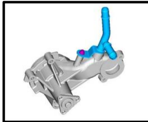
29. **(Single Alternator)** Install the supplied #2-113 oring to the shorter heater tube and install to factory location, secure with stock fastener, torque to 89 lbs-in. Reconnect both factory hoses, secure lower hose with stock clamp.
