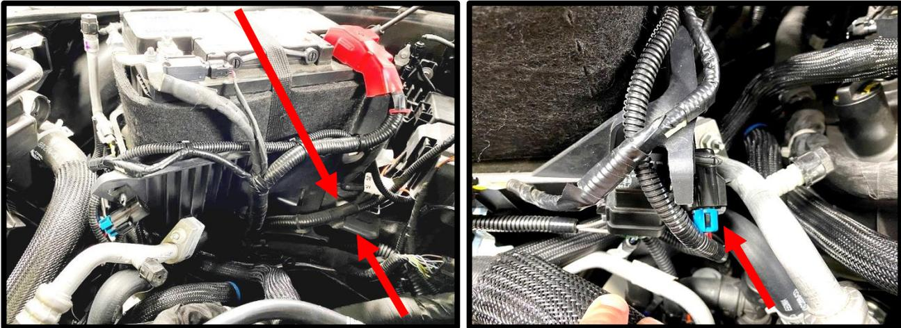
109. Using a 10mm socket, remove the nut on the power stud, located on the positive stud under fuse box cover. Install the IC pump relay power eyelet (red wire) to the power stud on the battery positive (+) stud. Use a 10mm socket to secure stock and IC power wire.
