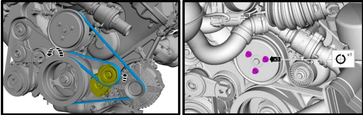
47. Using a 10mm socket, remove the (3) factory fasteners from the timing chain to head cover and (1) from water pump (for new idler plate).
