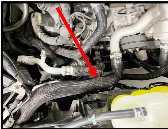
42. **(Dual Alternator)** Reconnect factory quick connect fittings to new coolant tubes.
