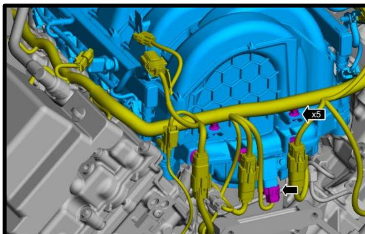
22. Remove the (4) bolts securing fuel rail to intake manifold. Lift rail up and away from manifold.
