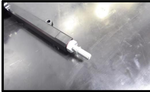
53. Install the stock injector pigtails to the fuel injectors. Install the supplied (4) fuel injector position lock brackets to clock the supplied fuel injectors into proper position. While installing the lock brackets, secure the fuel injector so it does not add pressure to the injector body. **Note:** This is for dual spray pattern injectors only that must be at the correct angle. **TIP: Failure to clock the injector correctly can cause severe running issues and motor failure.**
