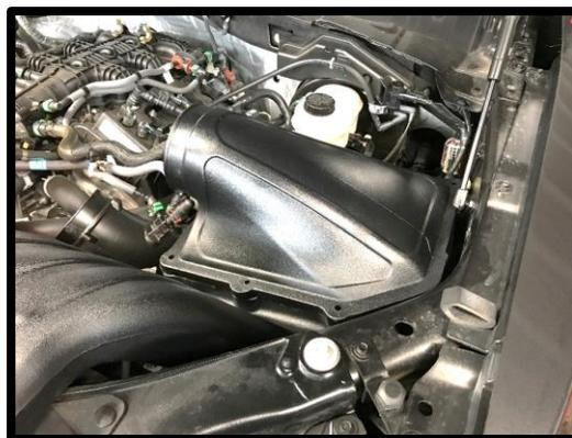
104. Install the (1) supplied 13/16" to 1/2" rubber grommet into the supercharger inlet tube. Install the supplied 1/2" to 15.82mm quick connect fitting.
