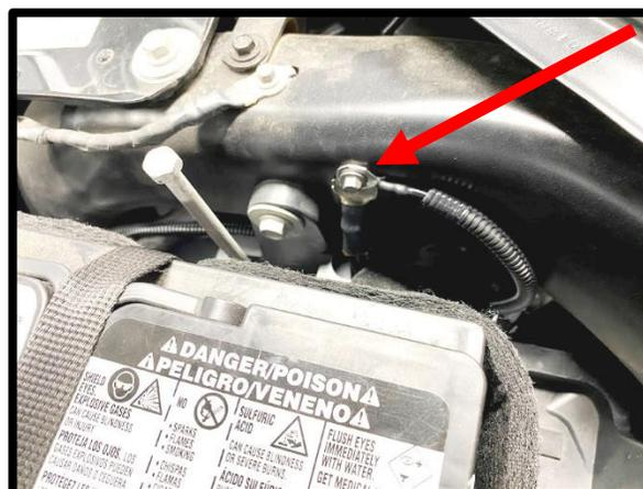
111. Pull the red 10amp fuse from position #F23 (ABS). Install the 10amp red fuse in the unused fuse slot on the fuse tap. Install the supplied fuse tap into position #F23 (ABS). **Note:** 10amp red fuse should be in bottom slot, 5amp should be in top slot. Make sure wire has enough room when fuse cover closes, route around fuses for clean installation.
