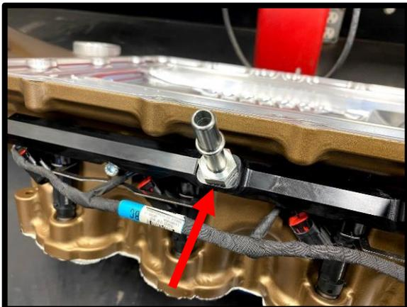
52. Install the supplied (2) #2-906 orings to the (2) inlet/outlet fittings. Install these (2) fittings into rear side of fuel rails. Apply light amount of grease to oring for ease of installation. Using a  $\frac{3}{4}$ " wrench (or  $\frac{3}{4}$ " deep socket) on both the front and rear fittings, tighten both.
