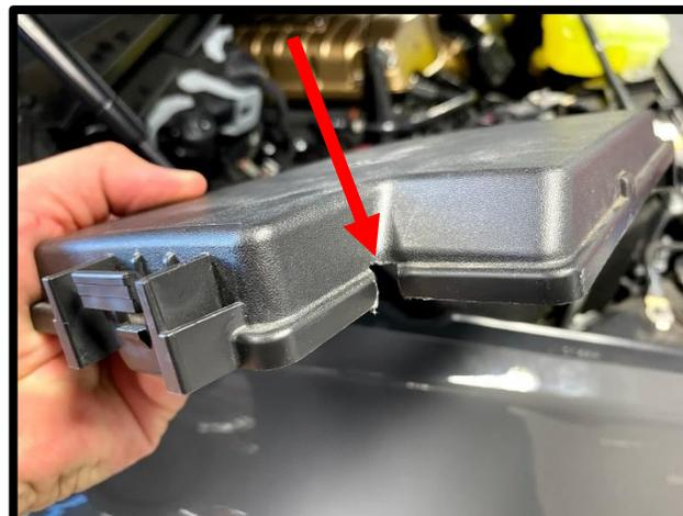
108. Locate the stock hole in the battery box as shown below. Use the supplied plastic push pin to secure the intercooler relay and fuse holder to the battery box. Route power and ground around box to fuse box area.
