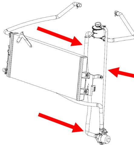
96. Install the 3/4" ID x 12" rubber hose (#3103092) from the **LH (OUTLET)** IC fitting to the IC filler neck. Secure both ends with supplied pinch clamps. This goes under the air inlet tube. **NOTE: NEVER SWITCH THE INTERCOOLER ROUTING, BANK 2 IS ALWAYS THE OUTLET!**
