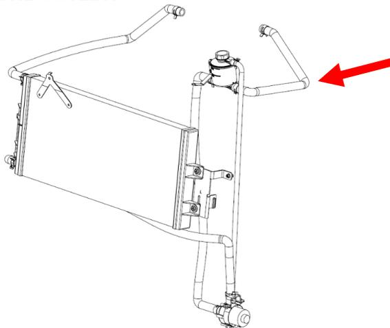
97. Install supplied  $\frac{3}{4}$ " ID x 22" hose #3103093 90deg end to heat exchanger top fitting. Route other end to **RH (INLET)** intercooler fitting. Secure with supplied constant tension clamps. **\*NOTE:** Make sure the hose does not and cannot kink during routing. **DO NOT** lay the hose on the cam sensor wires, this will lead to failure over time.
