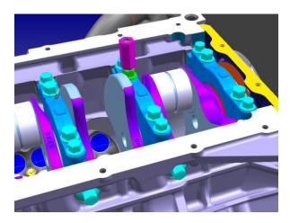
3) Install oil pick-up tube spacer on rear main studbolt and torque to 21-28Nm (17mm hex).
