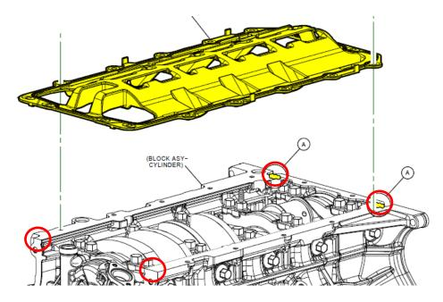
10) While holding windage tray up off cyl block, apply RTV dots in the 4 positions as illustrated above.
