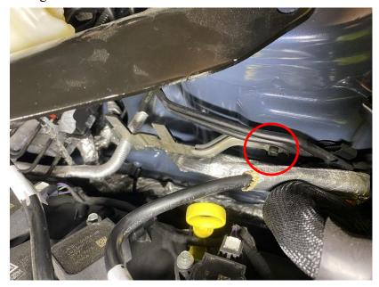
Step 8: Slide LH oil separator (CM-6766-M50D) onto bracket.
