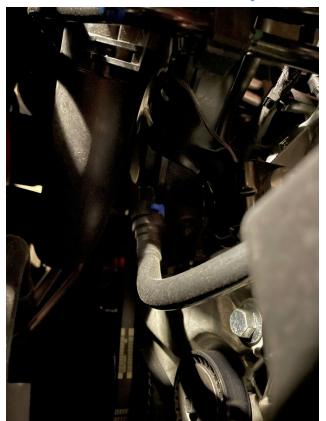
Lightly lubricate inner O-rings with engine oil and firmly connect lower PCV tube connector to induction tube spigot.
