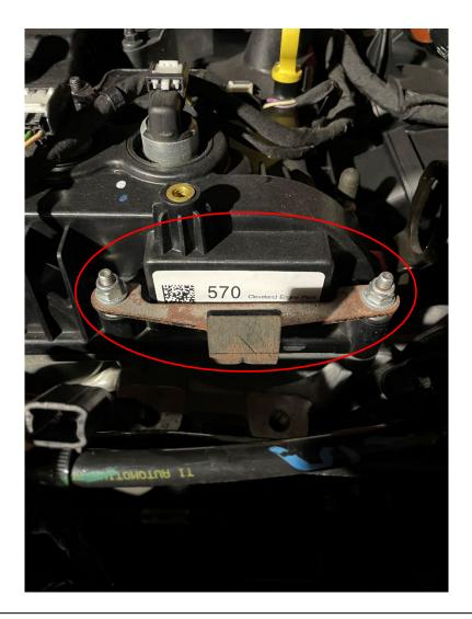
Remove vacuum line retainers from camcover studbolts, then install bracket over camcover studbolts and install (2) nuts. Torque to 10nm (88lbin).
