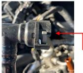
1) If your vehicle is equipped with the Orange colored connector, gently pry upward on the bottom of the connector (2 screwdrivers on either side work best) to break the connector from the camcover spigot. This breakage is normal as the connector is considered not serviceable.
