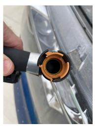
This removal will break the (3) locking tangs on the Orange connector. This is normal and necessary to remove the tamper-proof connector from the camcover spigot.
