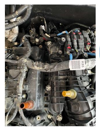
If your vehicle is equipped with the Orange colored connector, gently pry upward on the bottom of the connector (2 screwdrivers on either side works best) to break the connector from the camcover spigot. This breakage is normal as the connector is considered not serviceable.
