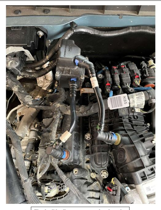
Firmly slide oil separator onto bracket tab. Lubricate inside of PCV connectors with thin film of oil and snap onto camcover, oil separator, and induction tube spigots. Make sure to install completely, looking for blue tab on connector to be locked.
