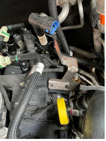
Install LH bracket using (2) W506856-S439 thread-forming screws and torque to 8.5Nm (75lbin). TIGHTEN BY HAND ONLY, DO NOT USE PNEUMATIC OR ELECTRIC TOOLS.
