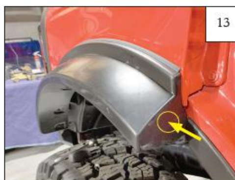
Use (1) SW1-0058 screw on end of flare.
