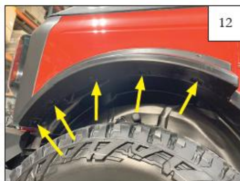
NOTE: Ensure that edge trim is seated correctly before proceeding. Press flares firmly onto the vehicle and install and fully tighten (5) SW1-0058 screws.
