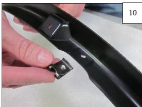
Verify presence of U-clip on inner brackets.
