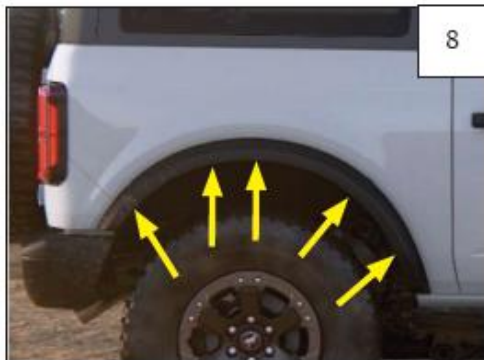
Twist (5) quarter turn fasteners. Firmly pull on flare to remove.
