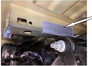
PROTECTIVE TAPE APPLIED ON THE REAR OF THE CROSSMEMBER ABOVE THE SPRING SHACKLE
