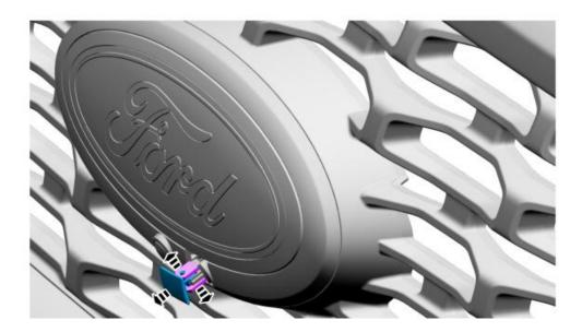
1.18 Remove the screws and the front camera washer and bracket as an assembly.
