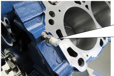
Oil pressure available at the right rear of block via -4 AN fitting with an O-ring seal. Note that fitting will need to be fabricated as shown. Oil pressure will read 10 lbs. lower than the pickup point at the left front port above the oil pump.
