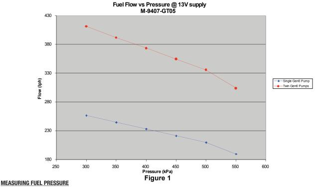
The above fuel pump sizing information should be regarded as a **guideline** in selecting the size of pump you need. Once installed in the car, you still need to **verify** that adequate fuel pressure (at least 39.15psi across the injector) is maintained at all engine speeds and loads. Do not skip this fuel pressure verification step, as failure to maintain adequate fuel pressure can cause issues ranging from calibration difficulty to engine failure due to running lean.
